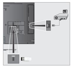
Connect the »USB1« socket of the television and the corresponding socket on the data device (external hard drive, digital camera, card reader or MP3 player) using a USB cable;
